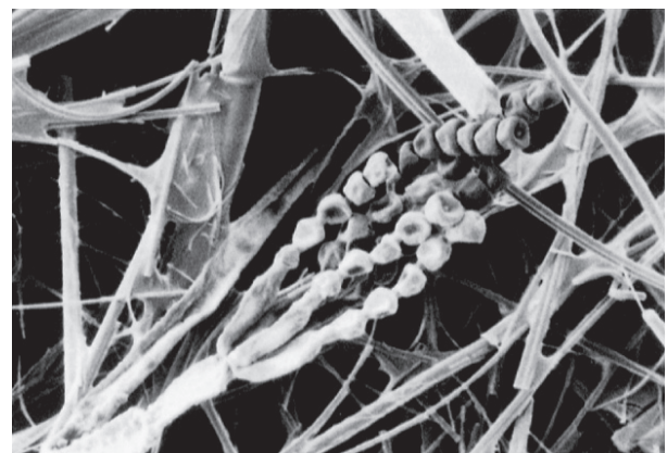
Fungus Build-Up on Conventional Filter
